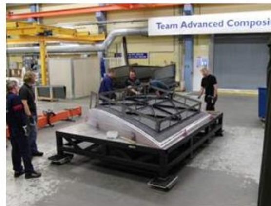
Current manufacturing of the Smart Wing integrated upper panel (SAAB)
